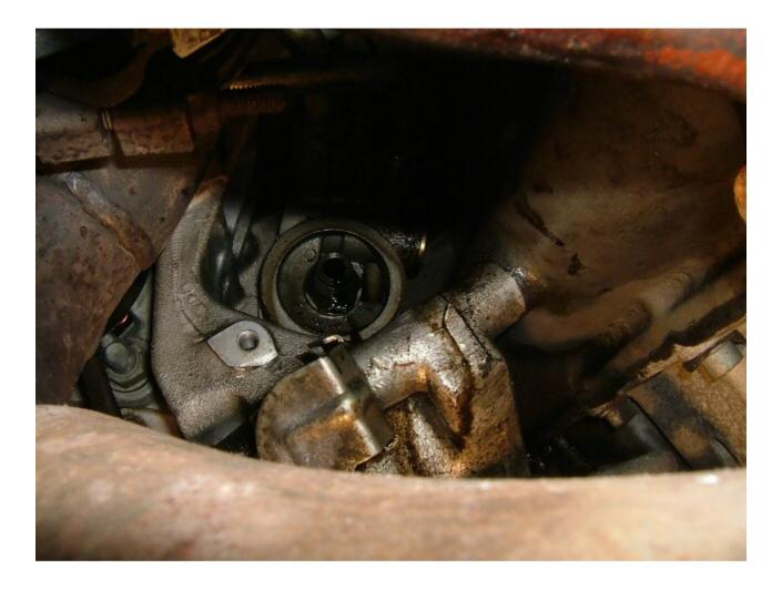
Before fitting the new *filter* pour a little fresh/clean oil into the lid of the oil can and smooth a thin layer of it around the rubber gasket on the new *filter* with your finger.
