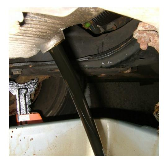
Leave for 10-20 mins to drain into the basin, then put a rag (or small plastic container) under the last of the drips and move the basin forward to catch the rest of the oil when you remove the *filter*, make sure it's under the 2 drain holes shown in the next pic.
