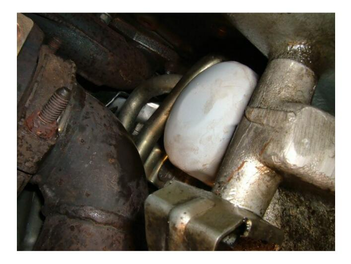
Refit the sump plug with the 8mm hex drive, but be VERY careful not to overtighten it as the thread is easily stripped!
