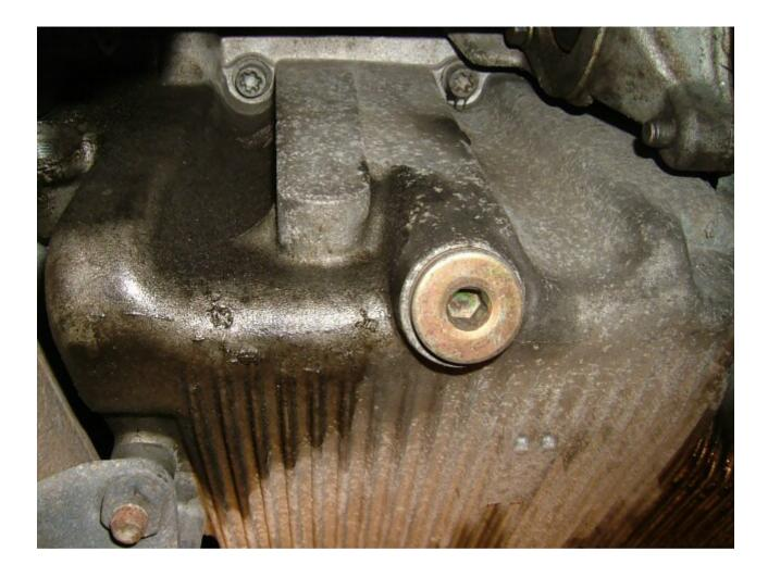
Place a suitably large basin (at least 5L) under the sump, as the next pic shows the oil flows out at an angle (not straight down) so make sure the basin is far enough back!
