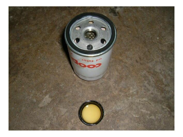
Tighten the new *filter* in place by hand, then use the wrench to give it a final 1/2 turn. The coupe is famous for leaking oil from around the *filter* so make sure it's tight, but don't over-tighten!
