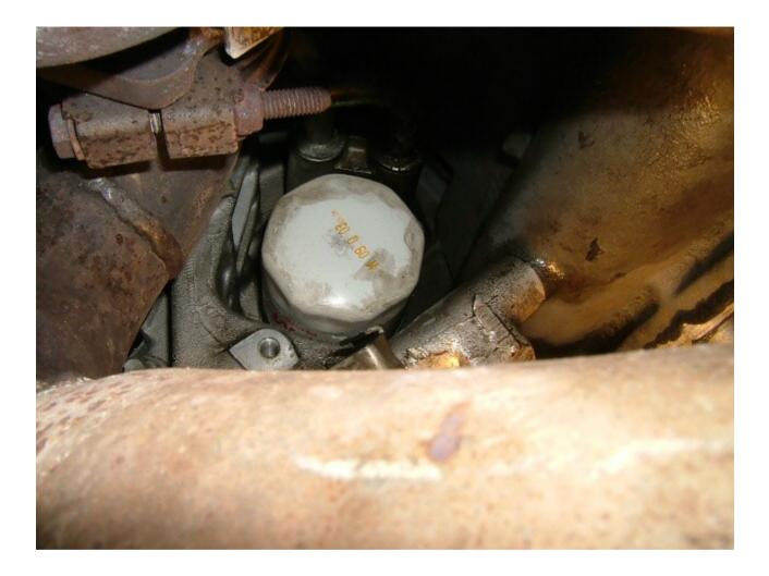
The standard *filter* is very short which makes it even more awkward to fit/remove. There's a suitable Champion *filter* F108 which is a bit *longer* but I couldn't source one of these anywhere locally so got another equivalent which was even *longer*, a Coopers Z68 *filter*.
